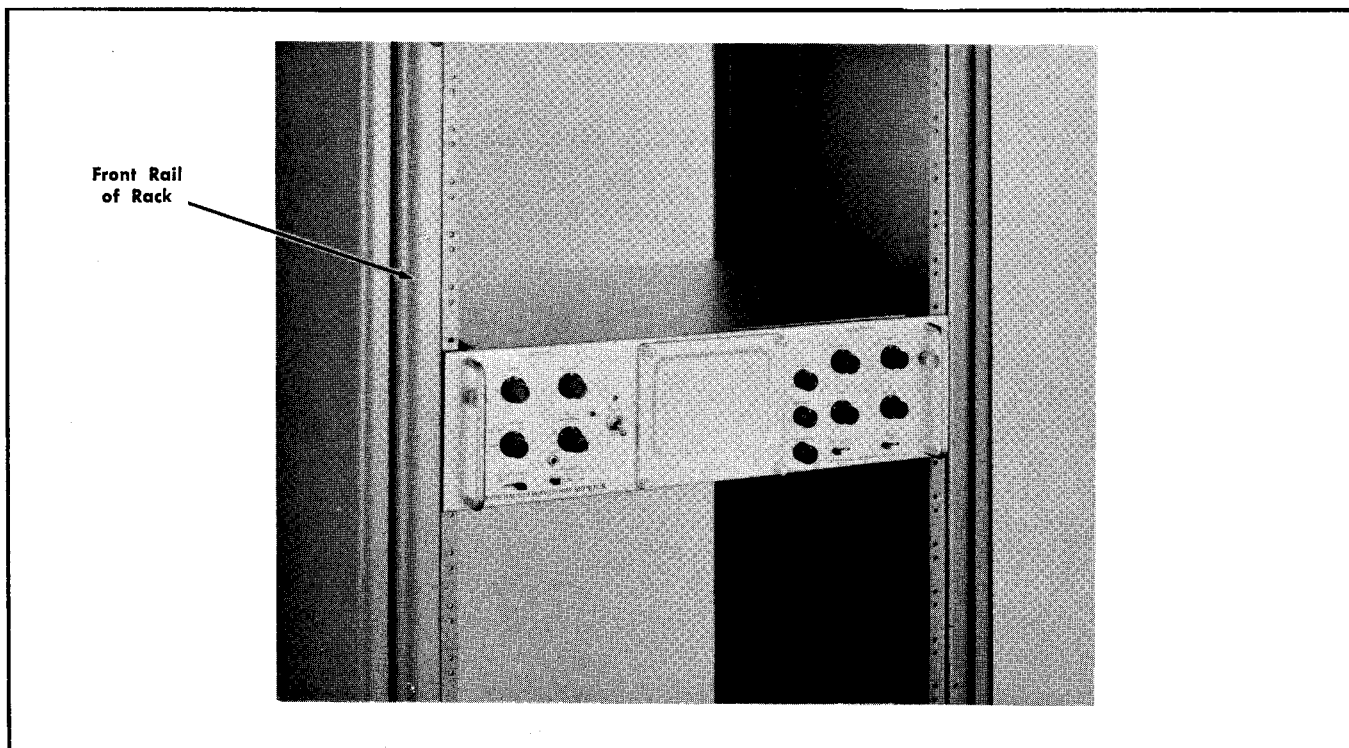
Fig. 10-1. The Type RM529 installed in cabinet type rack.
